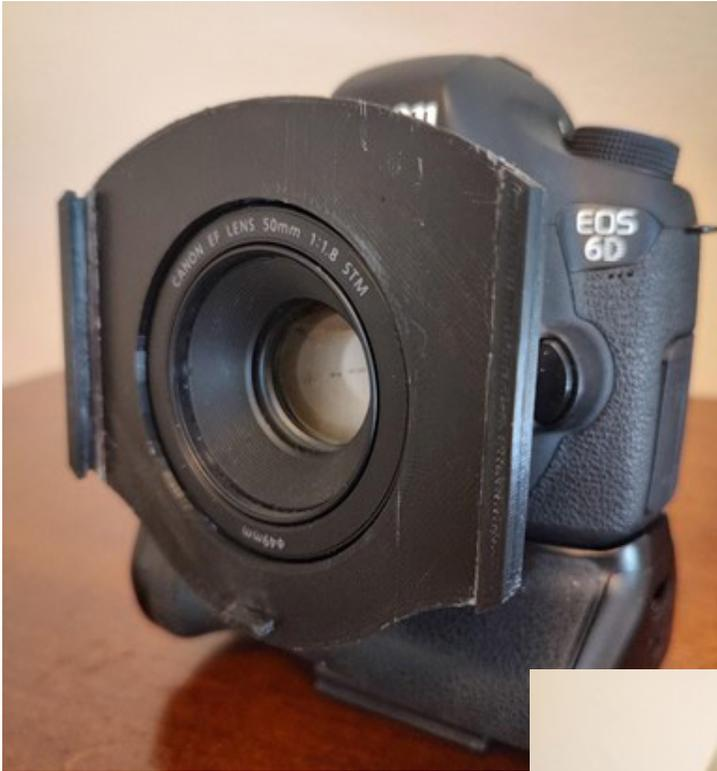
**CE Raum** created a filter holder for his 50mm Canon lens. I used the Prusa 3D printer to create two parts to very tight specifications, one part allows the filter to be easily slid in and out of the holder with no light gaps, and the back part locks onto the lens like an OEM part. After some light sanding the two parts were CA glued together. I will use this to shoot day-to-night timelapse.
