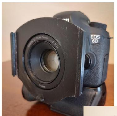
CE Raum created a filter holder for his 50mm Canon lens. I used the Prusa 3D printer to create two parts to very tight specifications, one part allows the filter to be easily slid in and out of the holder with no light gaps, and the back part locks onto the lens like an OEM part. After some light sanding the two parts were CA glued together. I will use this to shoot day-to-night timelapse.
