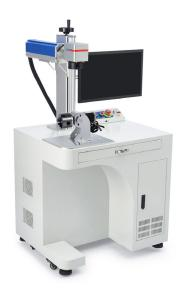
training. Also, very important, the fiber lasers are open systems. This means there is no cover like the CO2 laser have. So, safety is paramount. Safety glasses are a must. Also, if the laser can cut metal, it will cut fingers, so keep you hands away while operating the machine.
