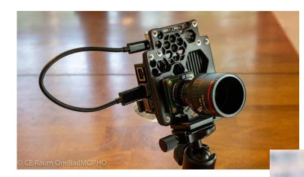
CE Raum used the Rasberry Pi HQ Camera, Google Coral USB Accelerator and Tensorflow TFLite software to create a camera that uses Artifical Intelligence / Image Recognition to capture images of birds at his birdfeeder.
