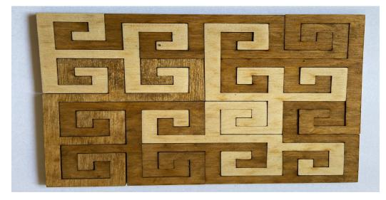
on the laser and stained selective pieces. It looks like one cut, but actually each piece is constructed individually, with allowance for kerf to get a snug fit.
